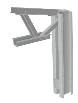
HINGED CONNECTION TO REINFORCED CONCRETE COLUMN
